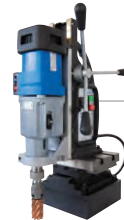
MAB 825 KTS p. 42 Capacity: \varnothing 3-1/8" cutter; \varnothing 1-1/4" twist drill; \varnothing 1-3/16" tapping Multi-axis positioning for boring, slotting, etc. Reversible, 4-gear motor
