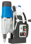
MAB 465 p. 36 Capacity: \varnothing 2" cutter; \varnothing 5/8" twist drill Reversible, 2-gear motor
